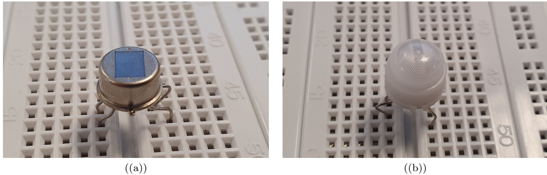
Figure 4: (a) Picture showing D4-323-AA Digital PIR Sensor. (b) Picture showing D4-323-AA Digital PIR Sensor with a fresnel lens on.
