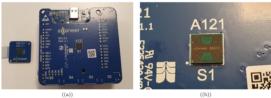
Figure 10: (a) Picture of the XS121 satellite board and XE121 evaluation board for the Acconeer A121 radar sensor. (b) Close up of the Acconeer A121 radar sensor.
